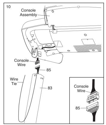
Set the console assembly on the Left and Right Uprights (82, 83). Be careful not to pinch any wires. Insert the excess wire into the Right Upright.
